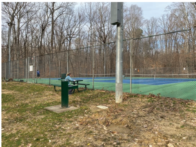
Amenities include benches and an accessible water fountain, located along the western edge of the court in complex 1; accessible route not provided to link ADA accessible fountain with courts
