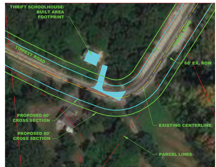
Draft diagram illustrating potential 60 foot road cross-section impact on Wyoming Farm (south) and Thrift Schoolhouse (north)
